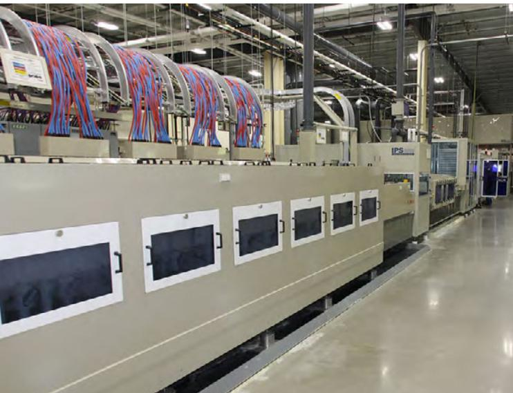
Figure 4: Horizontal pulse plater.
