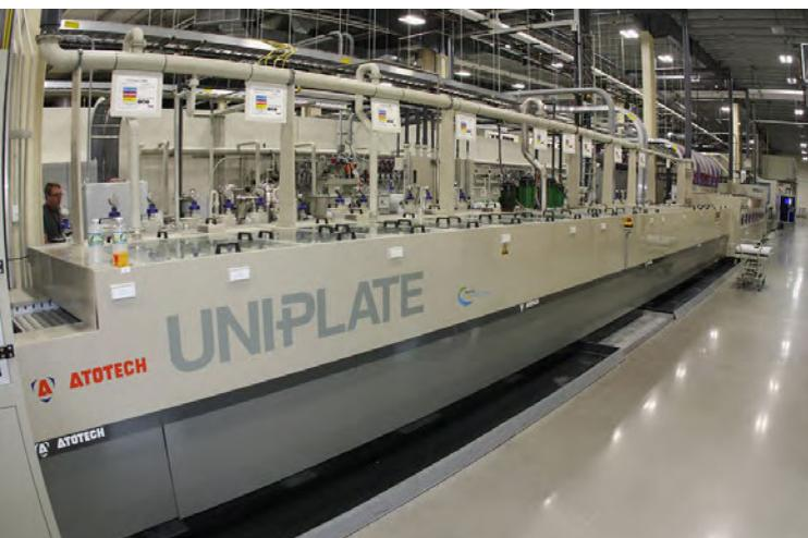
Figure 5: Horizontal conductive polymer process.
